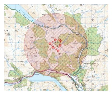
Figure 1: 4 km radius lighting activation zone around Kirkan Wind Farm<sup>2</sup>
